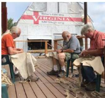
Virginia is also one step closer to sailing the seas with the near completion of her masts. Fred Gosbee and Stu Gillespie shape the spars with traditional tools such as axes, planes, and drawknives, as well as the good old traditional chain saw!
