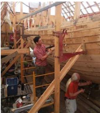
the work, which is nearly complete. MFS volunteers assisted Andros in his work, which included spinning the oakum and painting the finished oakum to prevent it from "walking out" and from leeching oil out of the seam compound, which will be paid over the seams.
