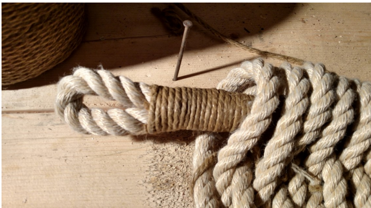
LEFT: An eye splice is "wormed" and "parceled" and ready for a tight wrapping of twine called "service."
