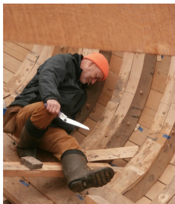
Photos clockwise from upper right: Orman Hines contemplates which side of the fo'c'sle he wants his bunk, portside view of Virginia, Roger Barry working on a shim, Dana Leonard fairing the inside of the frame.
