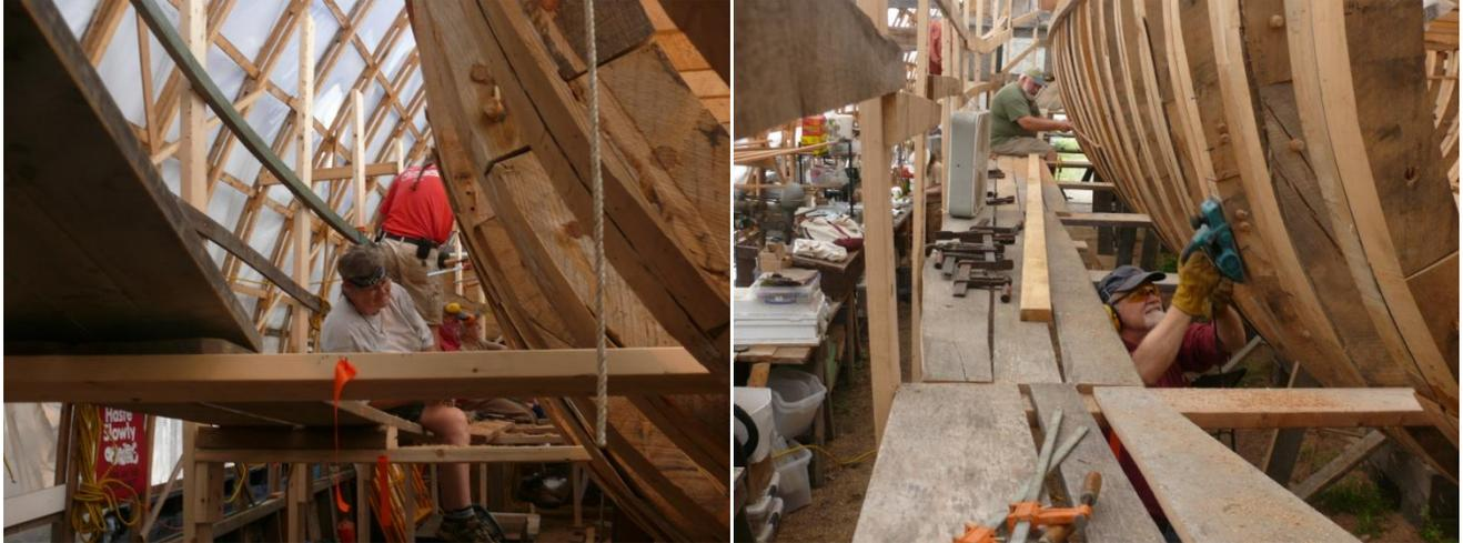
All fairing work now moves to the outer hull. Work continues from sheer to garboard to complete the preparation for planking. Above left, Gail, Jeremy, Tony and Chuck line up on the staging to apply planes and batten across multiple frames. While Dick applies shims and clamps (left)
