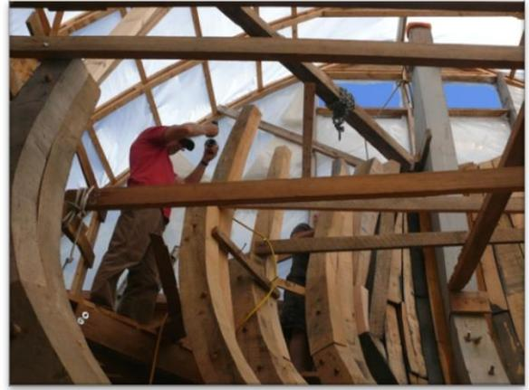
Les Perry (left) and Roger (center) work on some exterior touch up fairing, with the power planes. Roger Rand (right) drives the securing trunnel into the forward divided frame.
