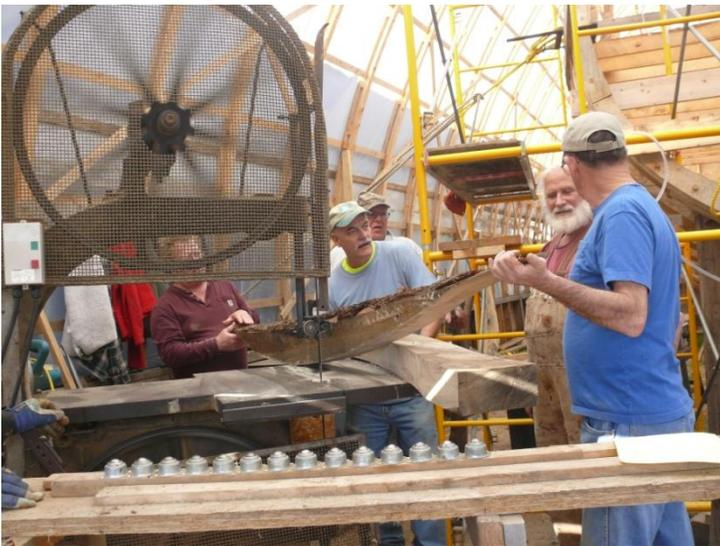
Finishing a cut, with the saw head at 90 degrees, Dick Forrest confers with Rob while removing the waste wood with help from John. You can really see the bevel and how it changes on the futtock that Roger is holding steady on the saw table. This functionality saves a lot of hand planning.
