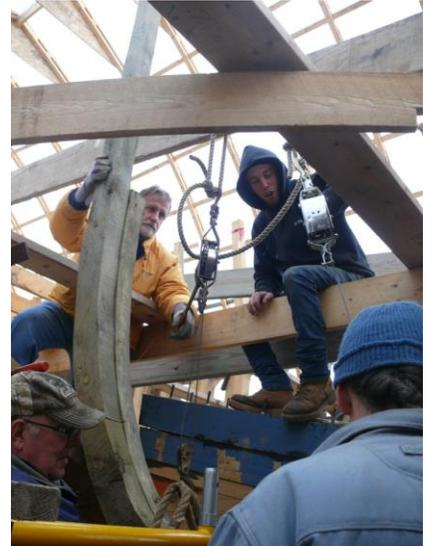
Once the frame is raised, Jeremy works from the staging to position and clamp the frame to the ribband while Paul guides the tenon end (below)
