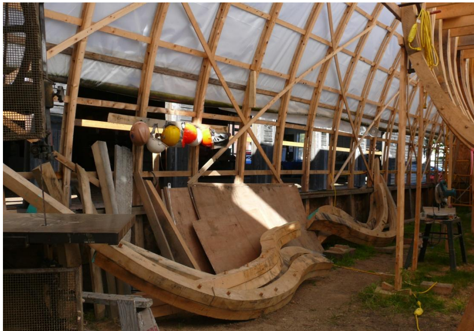
Aft frames #12, 13 and 14, arrayed in pairs, seem to share their graceful curves with the swept back wings of a diving raptor
