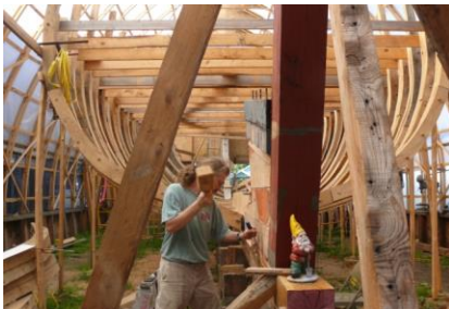
Tim Teague works on the changing depth of the rabbet as it rises higher on the deadwood
