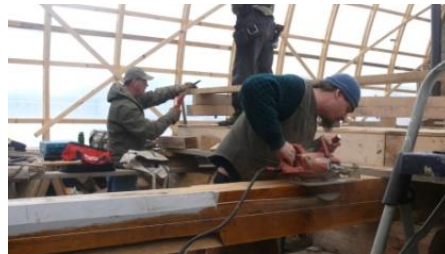
Jeremy Blaiklock cuts the keel rabbet using a circular saw preset to the correct angle.
