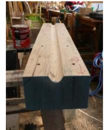
The nuts holding these stainless bolts are set flush with the top of the shaft log. The nuts holding the silicon bronze bolts are set flush with the interior of the shaft groove. Jay Coffey, Roger Barry and Tim Teague work (below left) on inseting the shaft log nuts.
