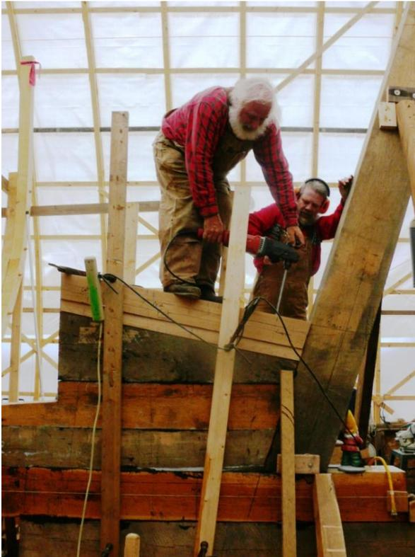
Standing on the stack of deadwood backing Virginia's sternpost Rob Stevens drills the 4 ½ foot, ¾ inch diameter holes that will receive the silicon bronze bolts which terminate inside the shaft log. Tim Teague repeatedly clears the drill shavings with the shop vac. Silicon bronze fittings are used to bolt timbers that will be under the waterline.
