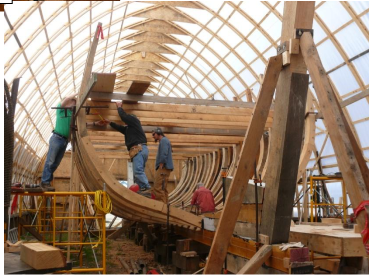
Above: Tim and Mark measure the diagonals from the horn to the plumb bob Jeremy has centered on the keel.
