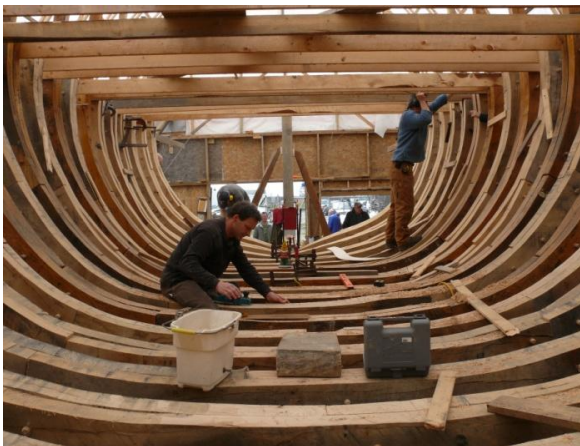
Above and Right: Jeremy and Gil laser sighting. Left: Bruce planes the center of each frame to fit the keelsons and Jeremy setting up for the plumb bob on the next frame to be horned.
