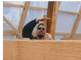
Above and Right: Jeremy and Gil laser sighting. Left: Bruce planes the center of each frame to fit the keelsons and Jeremy setting up for the plumb bob on the next frame to be horned.
