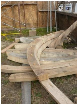
layout of each of *Virginia's* frames for assembly and drilling /inserting trunnels.
