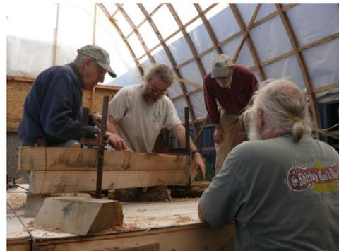
*Virginia's* forward frames are being built between now and May 2013 and consist of progressively beveled futtocks which are cut using the articulating ship's saw. As each futtock is milled, volunteers adjust the saw blade angle to engineered bevels as the cuts are made. Winter hours are Saturdays and Wednesdays from 9AM to 3PM. Visitors always welcome!
