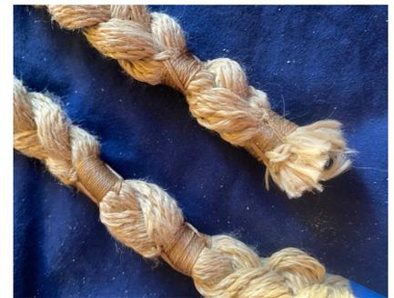
These are "lizards," which will be tied around the yards to make sure that the running rigging runs the way it's supposed to. You can see how the rope has been spliced around the bullseyes to keep them in place. The rope next to the bullseyes will then be "plaited," which most people call "braided." The smaller twine wrapped around the ropes forms "whippings" to
