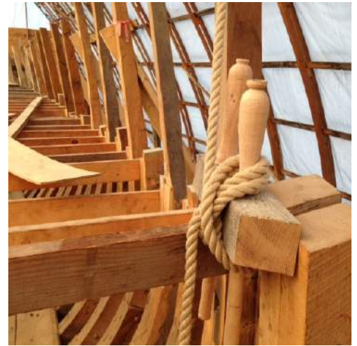
(Above) Belaying pins inserted into a prototype pin rail to refine the size and proportions for more than 50 production pins. (Below) Belaying pins turned from ash donated by Pat Maloy, and Dennis and Jane Menard. Photo credit: Steve Spaeth.
