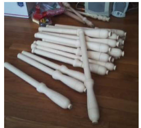
(Above) Belaying pins inserted into a prototype pin rail to refine the size and proportions for more than 50 production pins. (Below) Belaying pins turned from ash donated by Pat Maloy, and Dennis and Jane Menard. Photo credit: Steve Spaeth.
